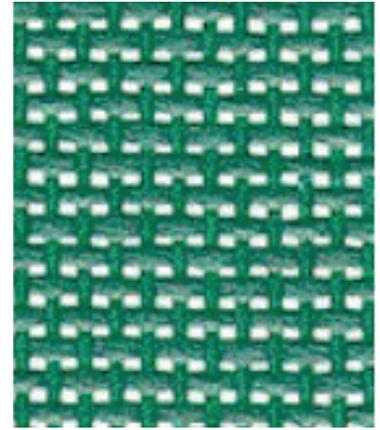
**Figure 8: Woven Mesh (23% void area)**
