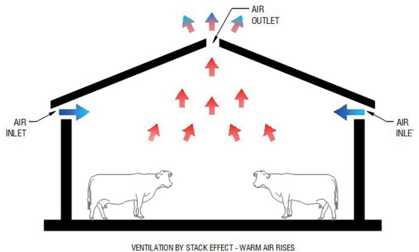
**Figure 1: Ventilation by thermal buoyancy**
