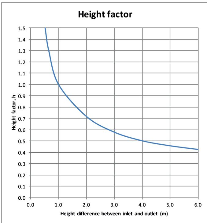
Figure 3: Height factor to account for difference in height between inlet and outlet
