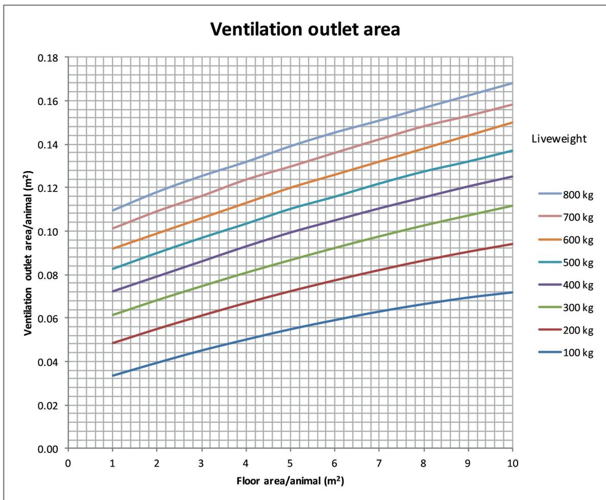
**Figure 2: Ventilation outlet area for cattle buildings where height difference between inlet and outlet is 1.0 m (see Figure 3 for height factor)**
