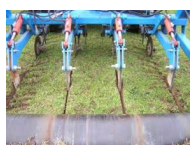
Roller for depth control and break back legs to reduce bringing stones to the surface
