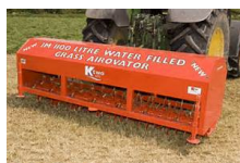
Spiker with water tank for extra weight
