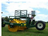
Roller spiker with grass seeder and frame for extra weight
