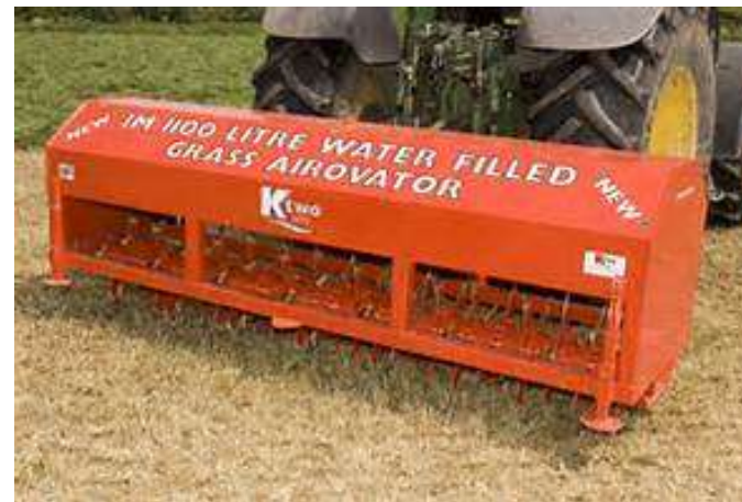
Spiker with water tank for extra weight
