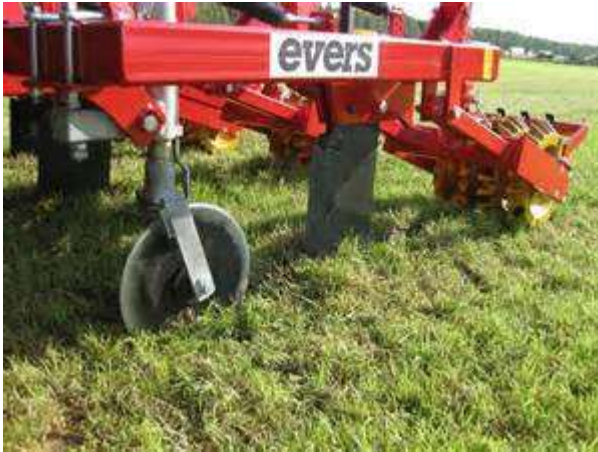
Pre-cutting Disc and Closer leg spacing
