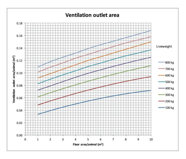
Figure 2: Ventilation outlet area for cattle buildings where height difference between inlet and outlet is 1.0 m (see Figure 3 for height factor)
