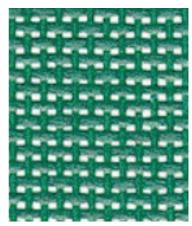
Figure 8: Woven Mesh (23% void area)
