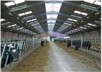
Figure 5: Ventilation outlets provided under central roof lights.
