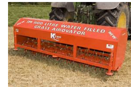
Spiker with water tank for extra weight
