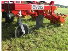
Pre-cutting Disc and Closer leg spacing
