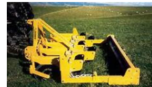
Roller for depth control and break back legs to reduce bringing stones to the surface
