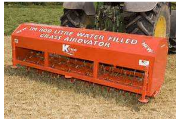
Spiker with water tank for extra weight
