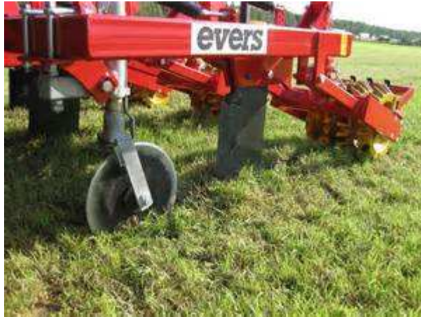
Pre-cutting Disc and Closer leg spacing
