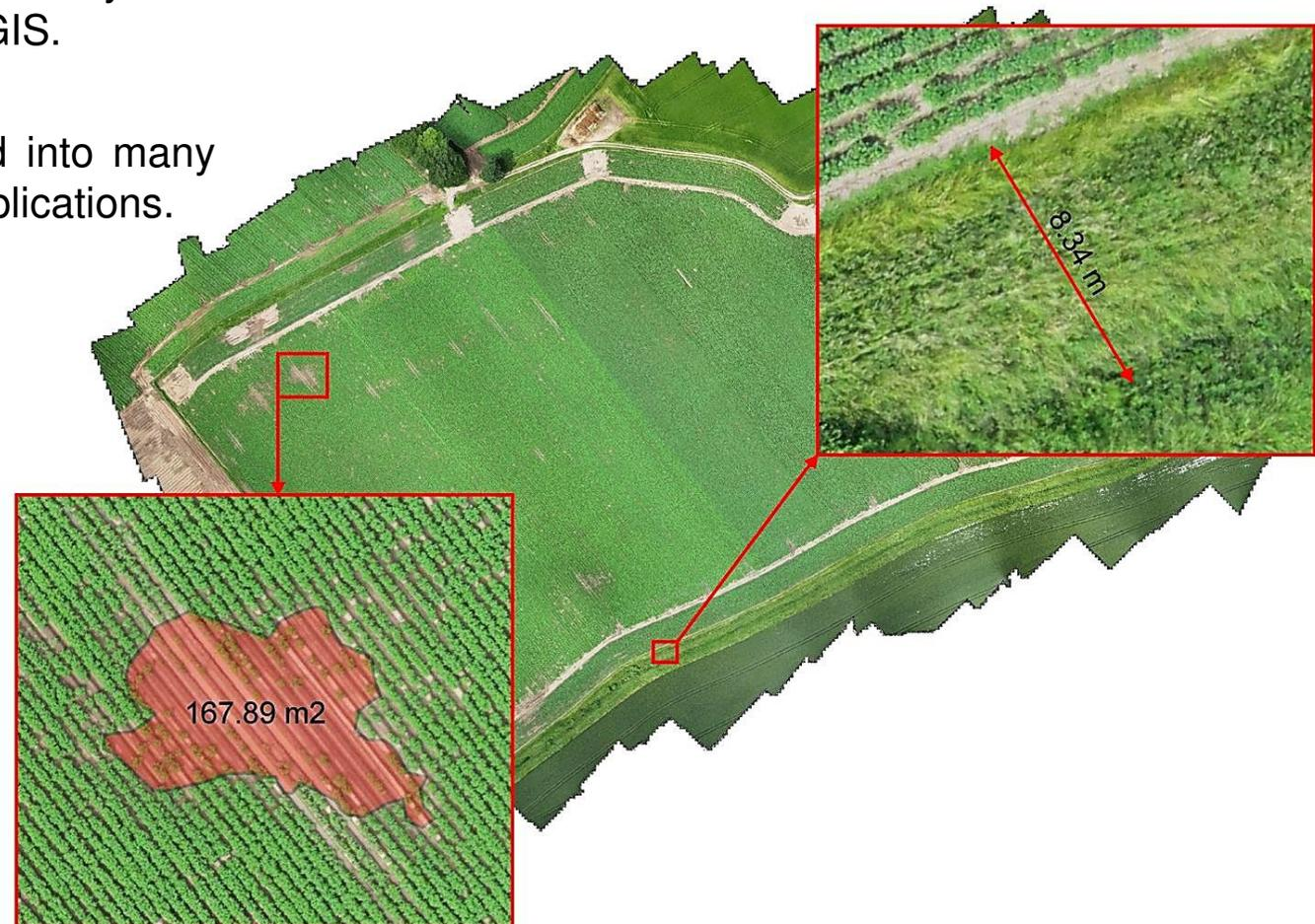
*(Measuring the area of a poorly performing patch in the field)*
