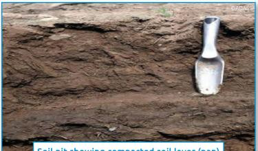
Soil pit showing compacted soil layer (pan)
