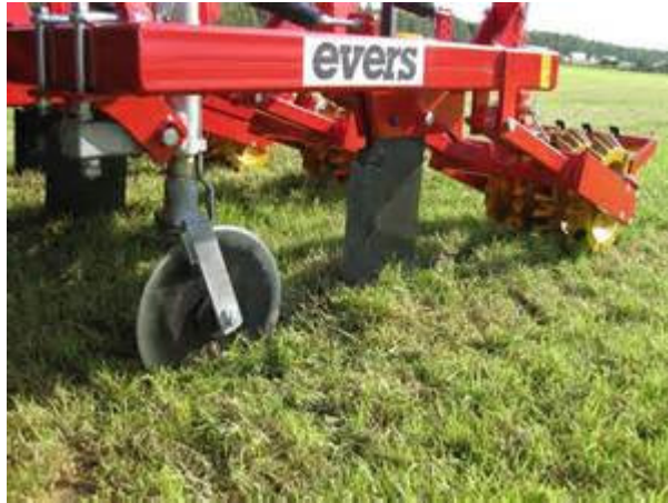
Pre-cutting Disc and Closer leg spacing
