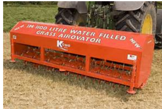
Spiker with water tank for extra weight
