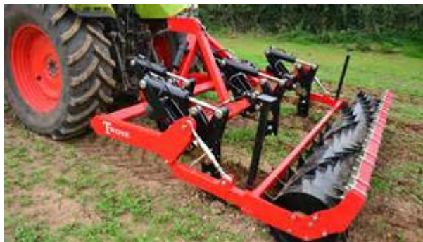
Spiked roller to help aerate surface
