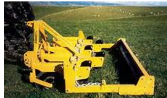
Roller to level surface following treatment
