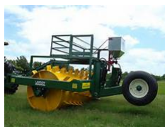
Roller spiker with grass seeder and frame for extra weights
