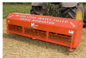
Spiker with water tank for extra weights
