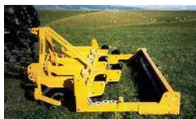
Roller to level surface following treatment
