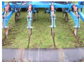
Roller for depth control and break back legs to reduce brining stones to the surface
