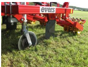
Pre-cutting Disc and Closer leg spacing
