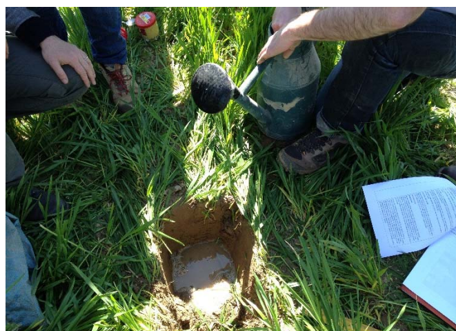
Figure 2: Mustard solution is poured into the hole and the infiltration is measured. Photo: D. Antichi
