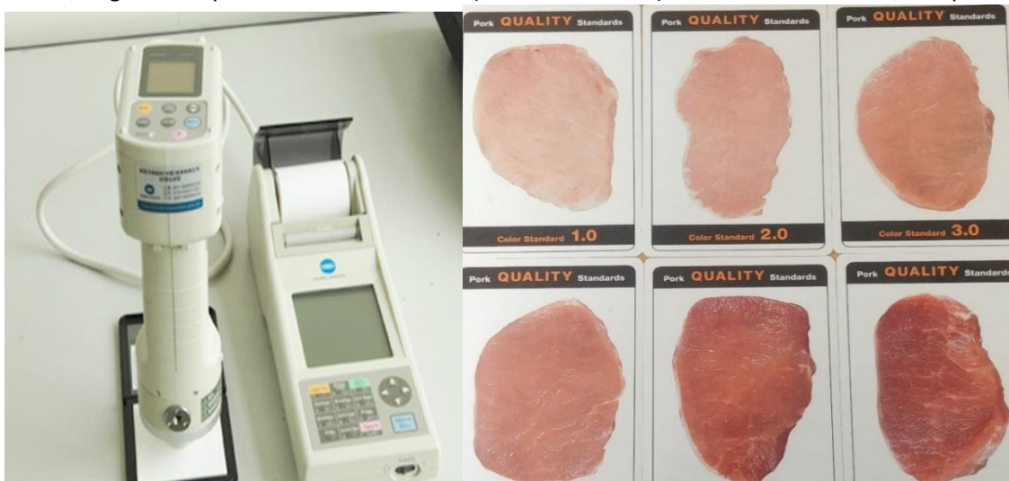
Figure 10. a) Koica Minolta CR-450. b) Colour standard cards from Pork Check off
