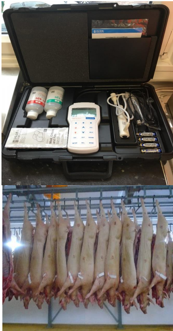
Figure 4. a) pH meter HI98163 b) Carcass tagged for meat quality sampling in differentiated rail in the commercial chiller.
