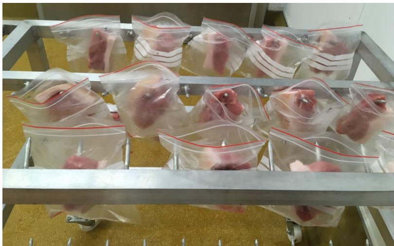
Figure 28. Drip loss samples with hanging method, used from 2019 onwards.
