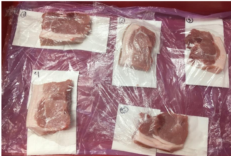
Figure 27. Drip loss samples with drip loss pads method, used until the end of 2018.
