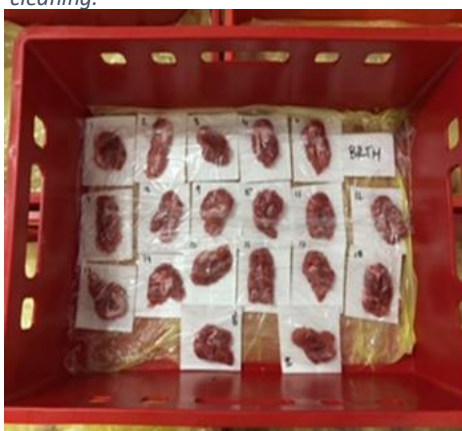
Figure 6. Samples labelled and placed in trades in commercial chiller for drip loss analysis.
