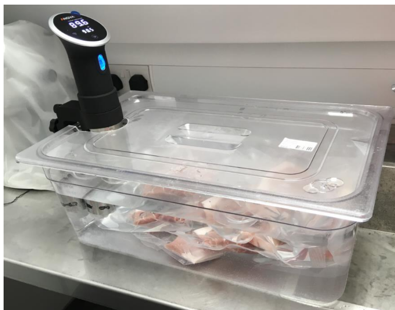
Figure 12. Thermostatically controlled water bath with meat samples.
