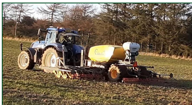
The System Cameleon drill / robotic weeder working in an organic oilseed rape crop growing in NE Scotland
