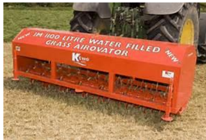
Spiker with water tank for extra weight
