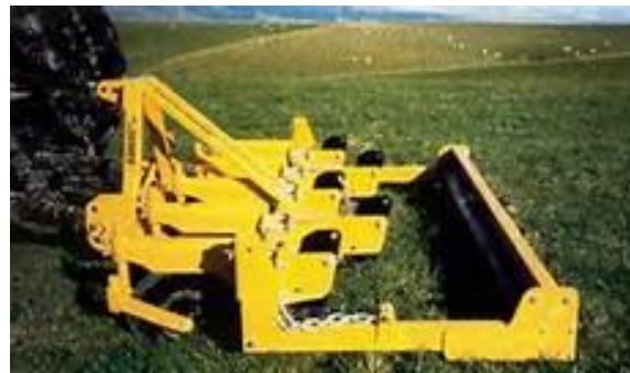
Roller to level surface following treatment
