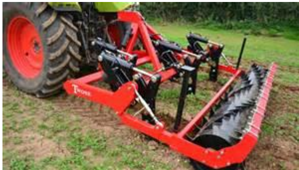
Spiked roller to help aerate surface
