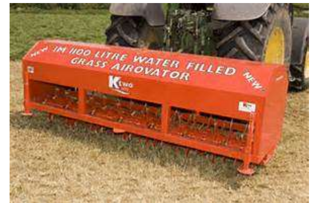
Spiker with water tank for extra weights
