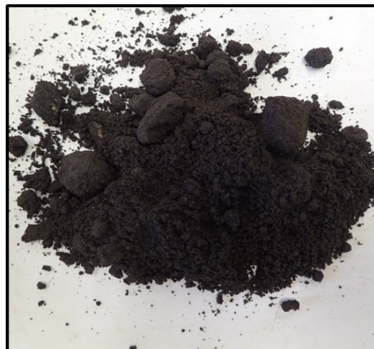
Figure 2: Sandy Loam with LOI of 5% and will have good rooting potential and nutrient management characteristics
