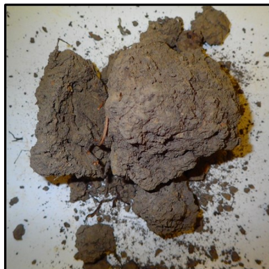
Figure 3: Clay loam with an LOI of 4% leaving it was a poor structure and drainage issue
