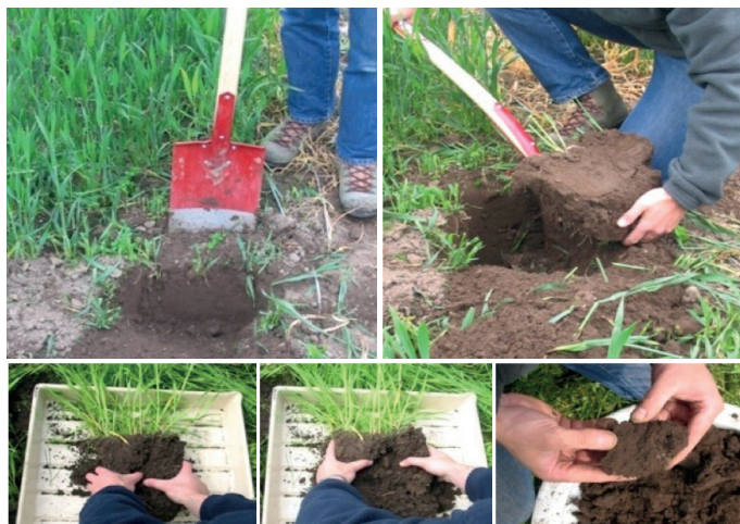
Figure 3. Sampling a block of soil for the VESS test.
