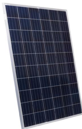
Figure 1: A typical PV panel would be 1.6 m long x 1.0 m wide x 35 mm and be rated at 0.25 – 0.45 kWp
