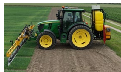
Figure 5. Skai Spot Sprayer mounted to the front of a tractor.
