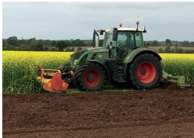
Fig. 4 Flail and rotavator combination © Bill Watts
