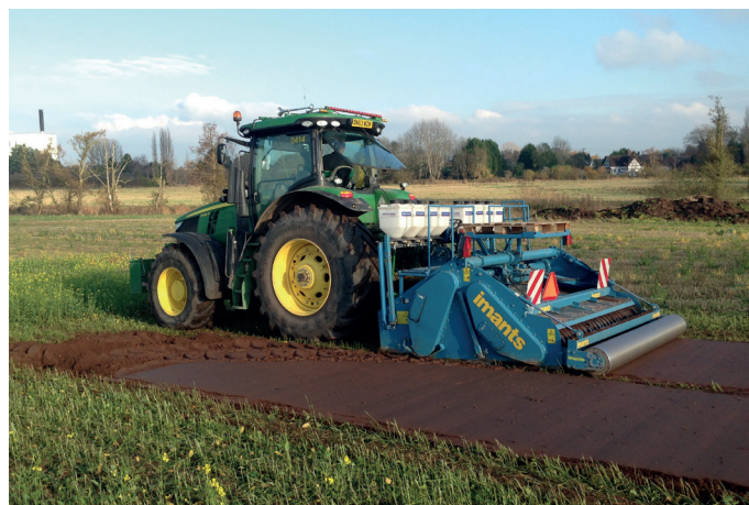
Fig. 5 Front mounted flail and rear mounted spader © Bill Watts
