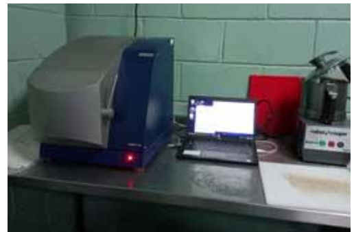
The FOSS™ meat analyser used to measure IMF%.
