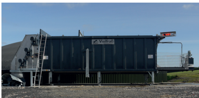
Figure 5: Feedstock intake hopper
