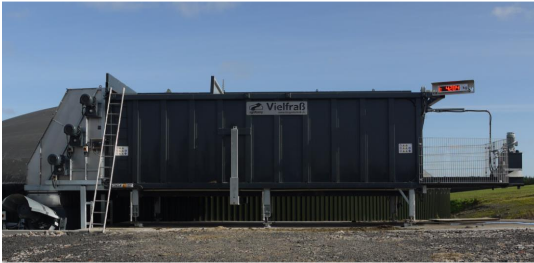
Figure 5: Feedstock intake hopper
