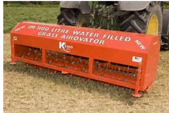
Spiker with water tank for extra weight
