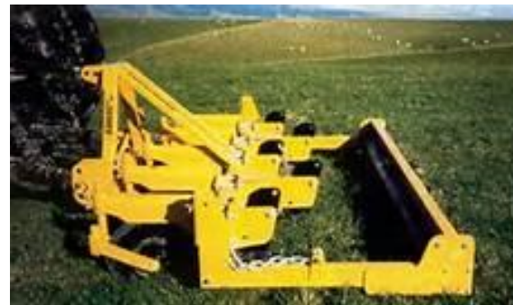
Roller to level surface following treatment
