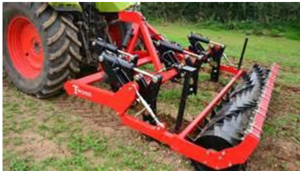
Spiked roller to help aerate surface
