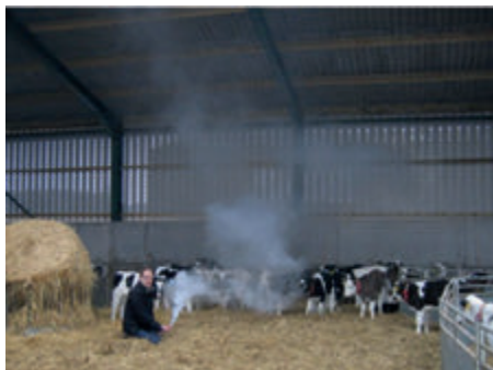
Use a smoke test to show the flow of air within a building
